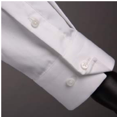
547L r'cuff folded angle bartack on the big side of sleeve pocket
