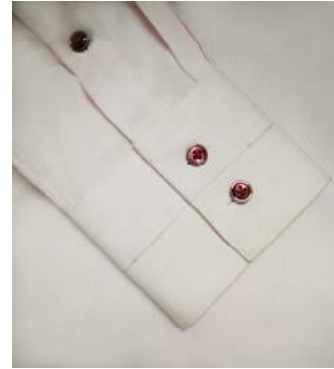
564L cuff band connection with hidden y shape pleat and bar tack
