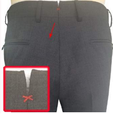
335C Back central seam V shape vent 3359 Red X stitching on V Seam on pant
