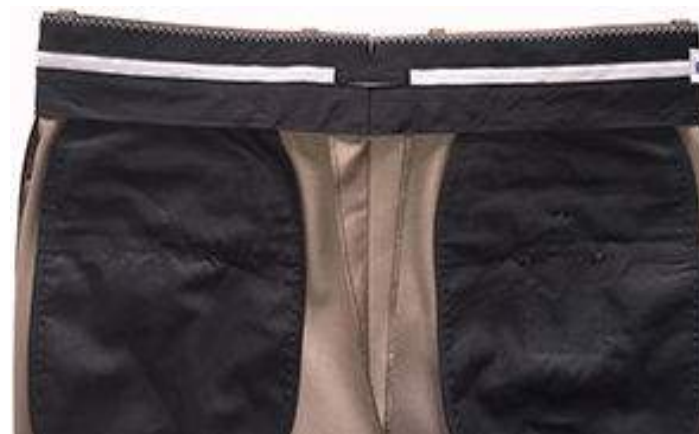
364Y Pocket lining in center of back waistband
