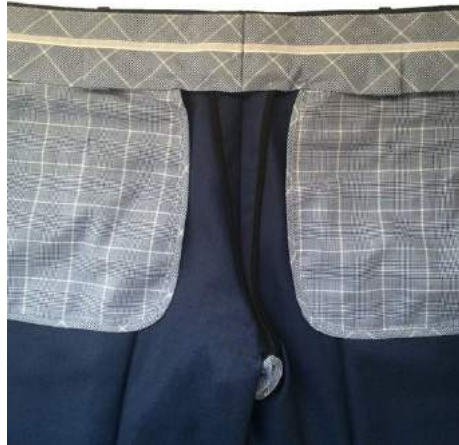
3521 Piping on back rise
