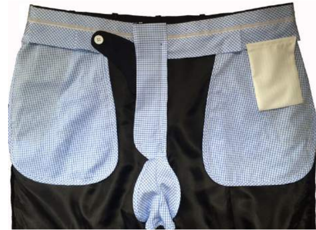
3147 reduce front pocketing depth by 4cm 3446 customer appointed materials for waistband pocket, pocket wrapping, under closure, small rise small rise piping and placket piping
