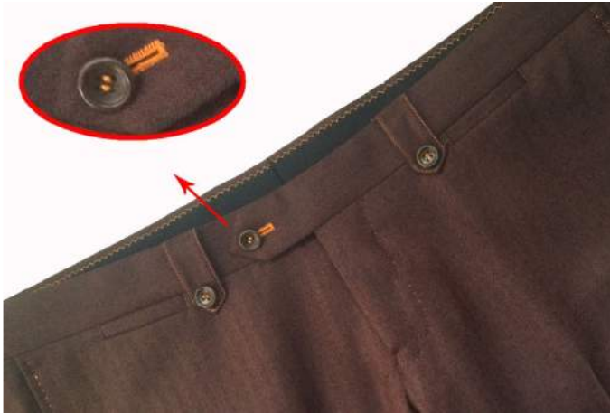
35DA Waistband buttonhole thread appointed 345H button thread match buttonhole thread
