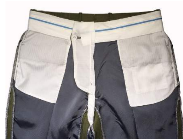
3523 net shape wrapping all used on side seam inner seam and back crotch seam
