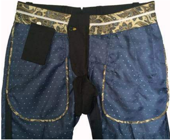
3144 add front pocketing depth by 2cm 35C1 Pocket fabric-customer appointed 35B9 pocket piping customer appointed fabric
