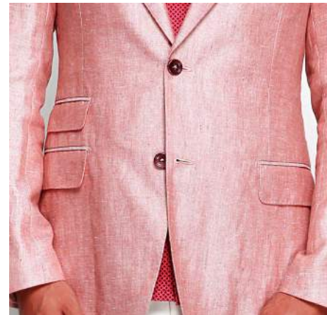
03B5 ticket pocket flap width 3.8cm, the split distance between ticket pocket and below pocket is 6.5cm 0202 Normal lower pocket and ticket pocket
