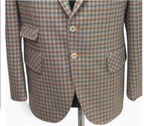
0917 the position of the bottom pocket raising 2.0cm 03C3 pocket flap width 7.0cm 03K5 45°slope-cutting external bottom flap 0202 Normal lower pocket and ticket pocket
