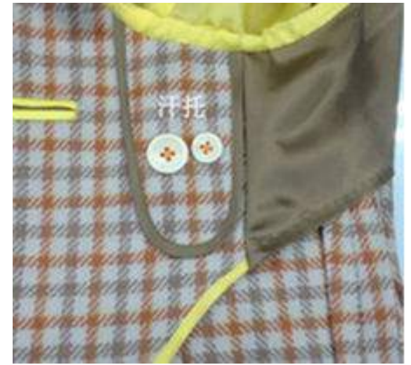
074P Right sweat pat with one large and one small button 0756 U Shape lining sweat pad with lining piping (L:11.5cm W:6.5cm)
